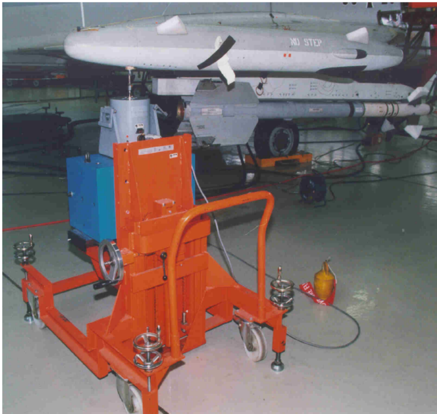
Figure 10: Mode Excitation on wing tip pod.
