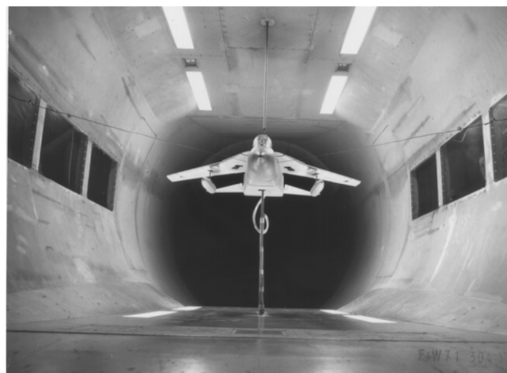
Figure 16: Aeroelastic Wind tunnel Model with external Stores underwing.
